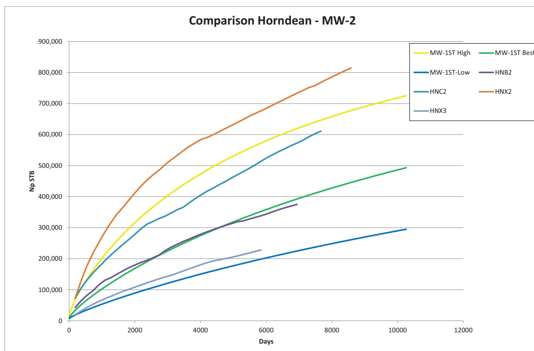
Figure 9.18 Comparison of cumulative production for the MW-1ST cases with the Horndean wells
